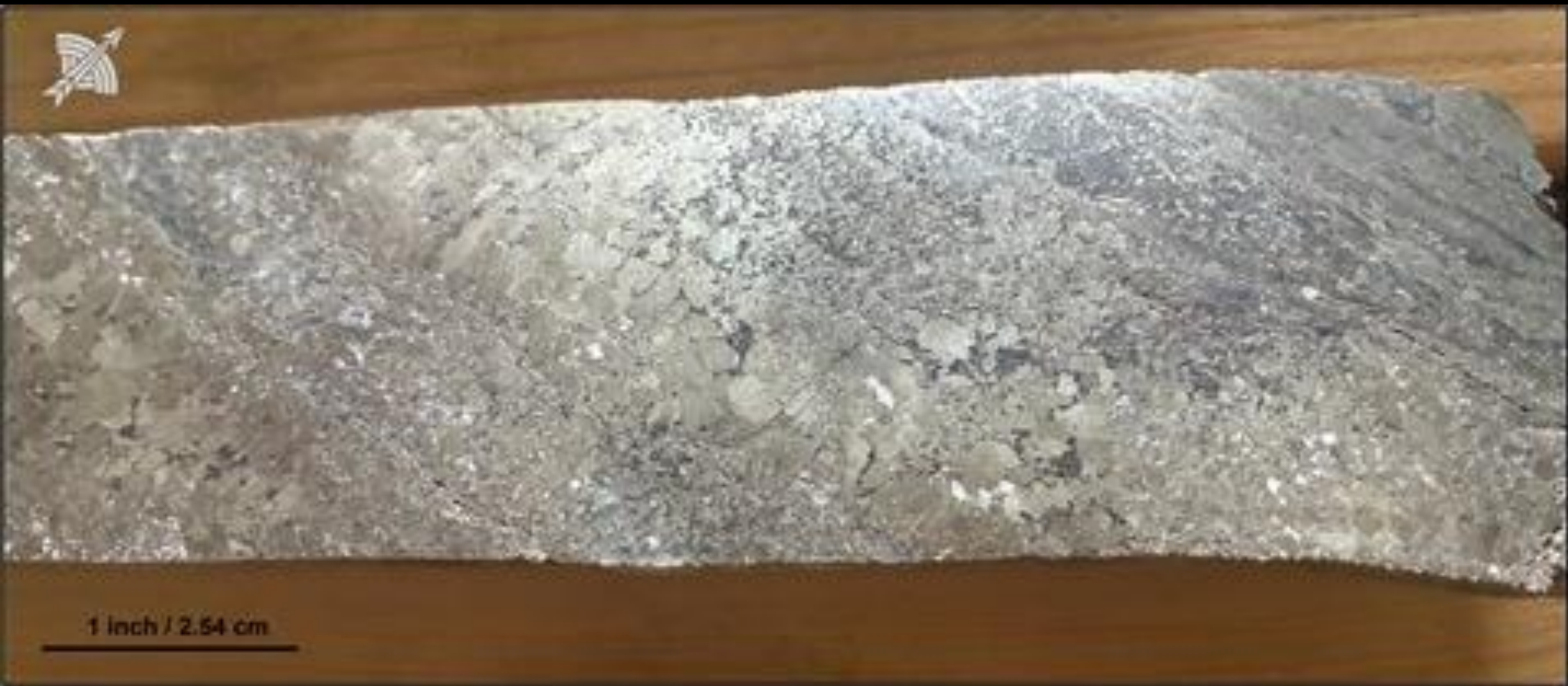
Figure 4-1 – Massive pyrite with chalcocite-bornite-chalcopyrite from DDH SBM26-09, Black Rock Copper Vein, at a downhole distance of 662.3m (Silver Bow press release, September 21, 2026).
