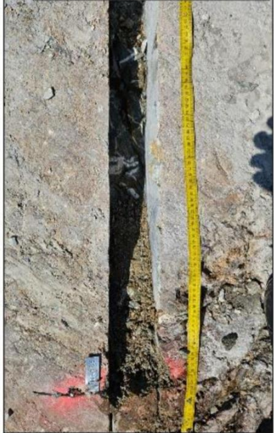
A ST112963: 0.73m Channel Grab Stockwork Quartz-Chalcopyrite-Sphalerite-Galena
