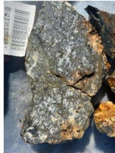
Samples from brecciated shears and veins with massive chalcopyrite and pyrite
