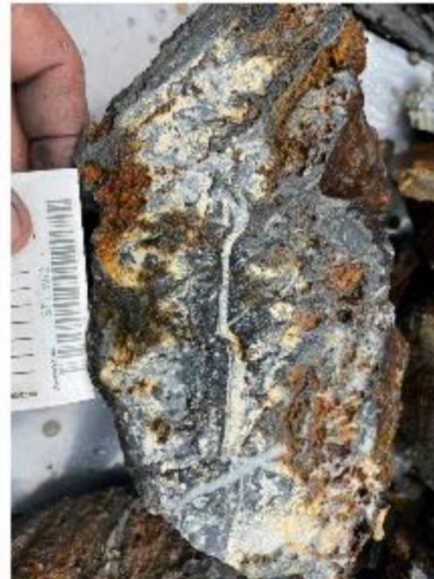
Samples from brecciated shears and veins with massive chalcopyrite and pyrite
