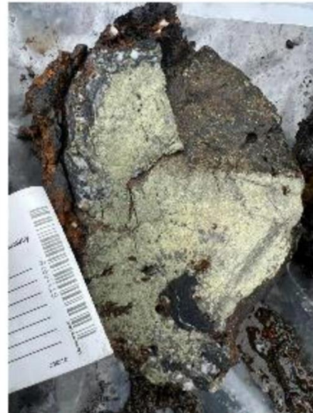
Samples from brecciated shears and veins with massive chalcopyrite and pyrite
