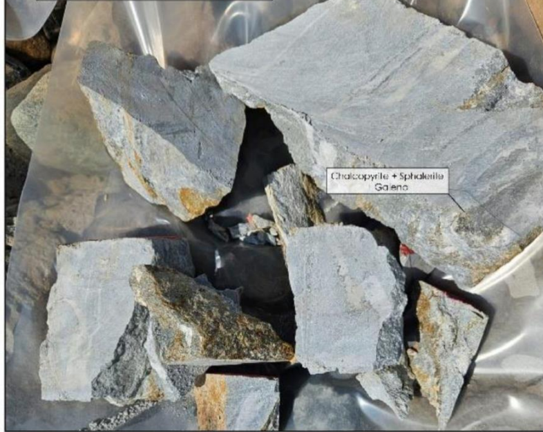
B ST112963: 0.73m Channel Grab Stockwork Quartz-Chalcopyrite-Sphalerite-Galena
