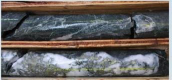
Chalcopyrite+pyrite mineralization in KLI-21-037 at 121 m
