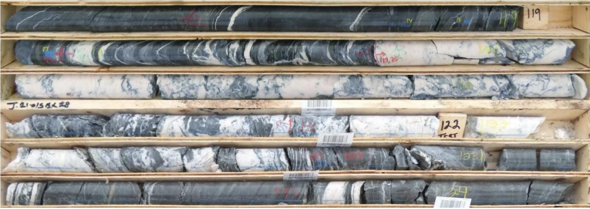
Figure 7 – J-21-015, collared 153m north of J-21-011 (see Figure 1), intersected a strongly mineralized quartz breccia vein nearly perpendicular to core across 2.95 m, with fine to acicular arsenopyrite mineralization in disseminations and along stylolites. View shown is from roughly 118.0 m to 124.2 m downhole. Assays for this hole are pending.
