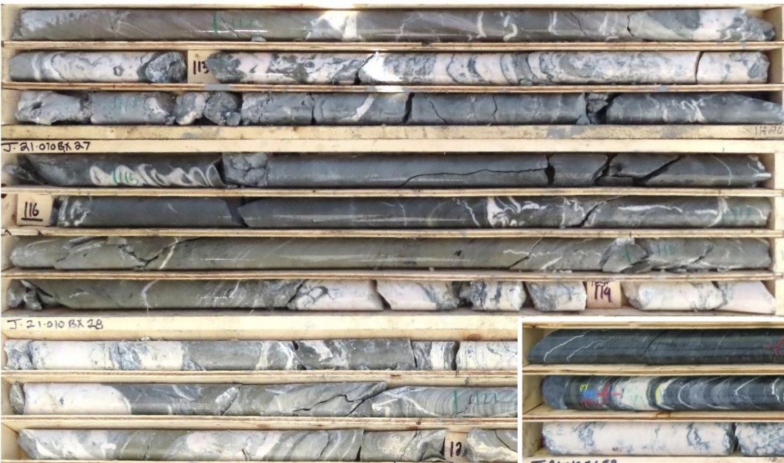
Figure 5 – J-21-010, drilled from the same pad as J-21-011, also intersected wide breccia, with patches of pyrite and arsenopyrite-bearing stylolites. View shown is from roughly 118.0 m to 124.2 m downhole. Assays for this hole are pending.
